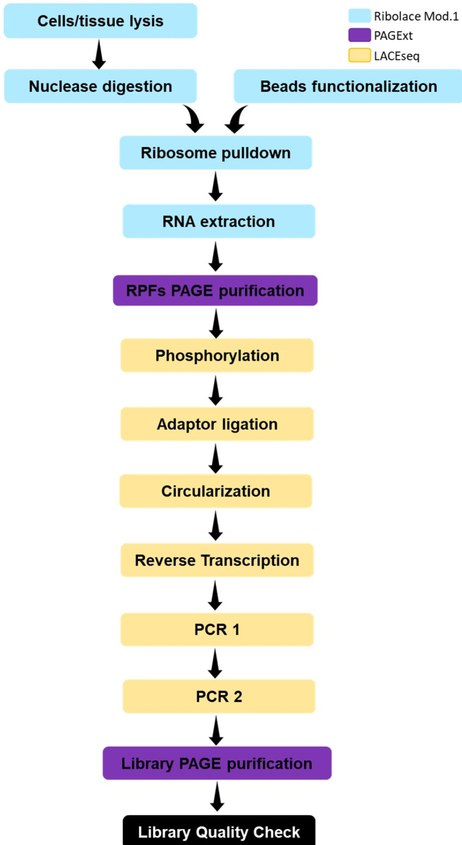
Figure 2. Overview of the Ribosome Profiling All-In-One Set workflow.
